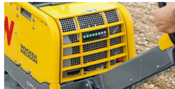
Compatec compaction control shows the operator when the best possible compaction has been achieved with this machine. This saves excess passes and time.
