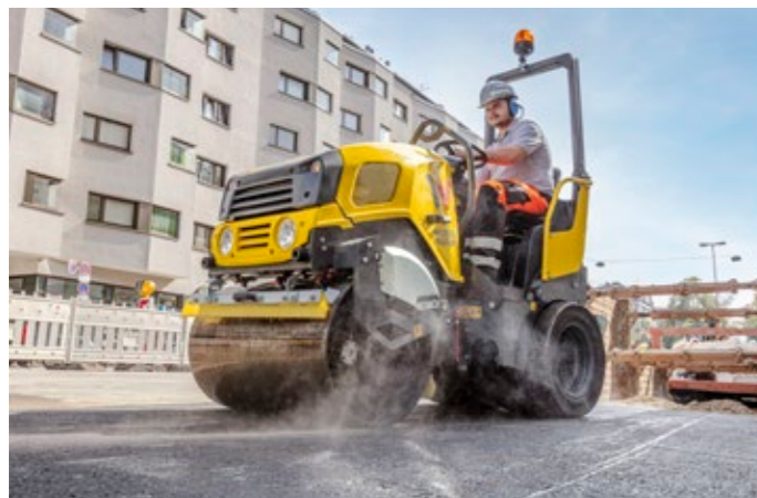
Tapered design for an unobstructed view of the drum edges, the machine surroundings and the construction site.
